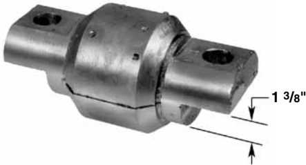
FRONT BEAM BUSHING OFFSET
